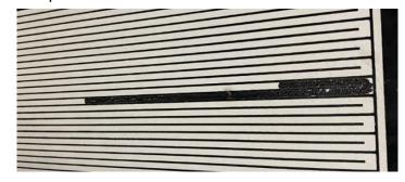
failure the resistive element will appear glassy/shiny compared to the gray metallic material that comprises the element. This is because porcelain material is similar in property to glass. If it gets hotter than it would during normal function, the heating element will attain the glassy/shiny look.
