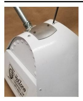
Disconnect power. Remove 2 screws that attach the element 'sled' to the housing.
