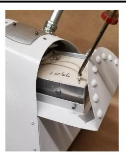
Disconnect leads from old element. Save the hardware for re-connecting your new element. If hardware needs to be replaced, use high temperature rated hardware (>900°F).
