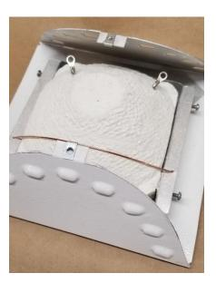
Remove old element from 'sled' and discard Install new element.
