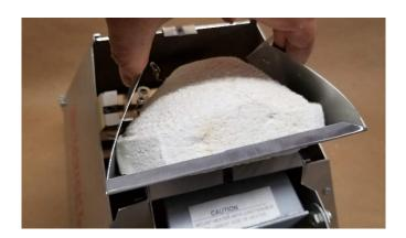
2. Install the new element. For the 1500W element: you may have to squeeze bracket legs as shown. Align bracket tabs so they hang over the housing attachment holes.
