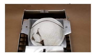
3. Attach the power supply leads to the element leads using the original screws and nuts and insulation
